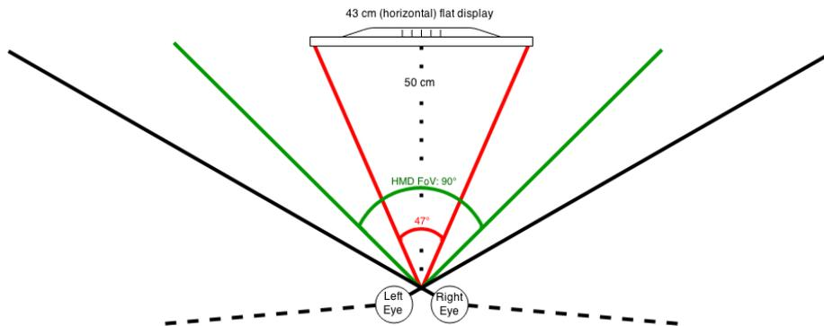
**Fig. 2.** Field of view offered by a HMD compared with a single traditional 43 cm wide display at a viewing distance of 50 cm
